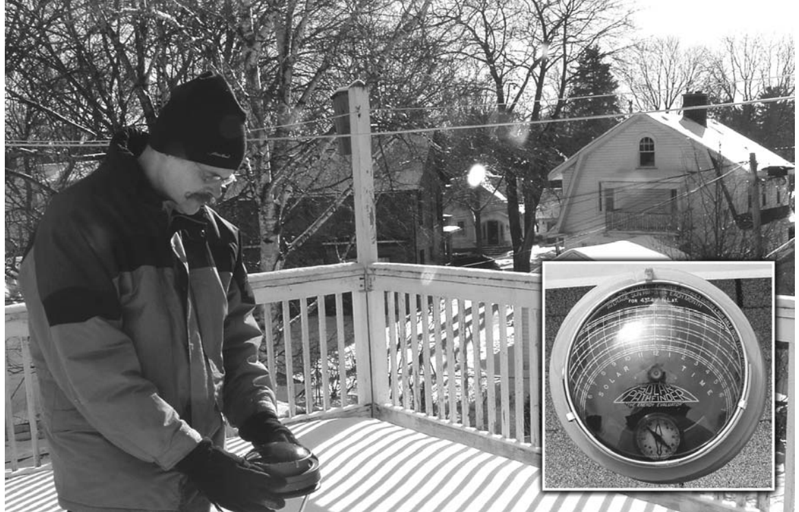
A site assessor uses a solar pathfinder to determine the effectiveness of solar energy at this home before the homeowner invests in a solar electric or solar hot water system. The inset photo to the right shows the Solar Pathfinder under ideal conditions.
